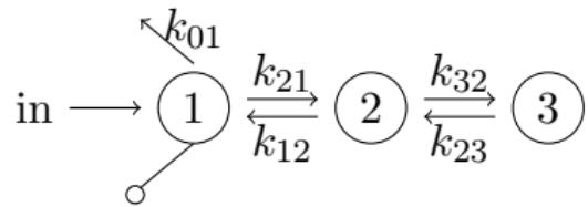
$$\begin{aligned} & y_1^{(3)} + (k_{01} + k_{12} + k_{21} + k_{23} + k_{32}) y_1^{(2)} \\ & + (k_{01}k_{12} + k_{01}k_{23} + k_{01}k_{32} + k_{12}k_{23} + k_{21}k_{23} + k_{21}k_{32}) y'_1 + (k_{01}k_{12}k_{23}) y_1 \\ & = u_1^{(2)} + (k_{12} + k_{23} + k_{32}) u'_1 + (k_{12}k_{23}) u_1 . \end{aligned}$$
